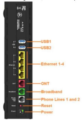
**IP Passthrough** means the Broadband CPE device terminates the VDSL/Fiber connection, authenticates with the network, receives a WAN IP, and shares that IP address with a single customer device connected to the Broadband CPE equipment. IP Passthrough will only allow one connection to be "unfiltered" or pingable from the WAN or internet side of the Broadband CPE equipment.
